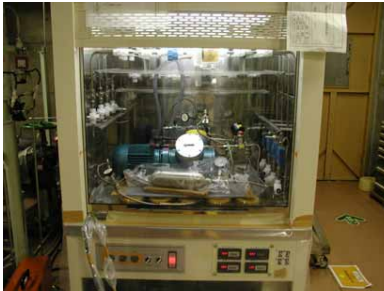
Figure 12 Sampling system of dissolver off-gas.
