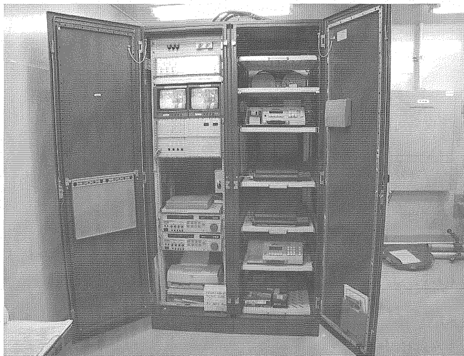
Fig. 3.3 Cabinet contained the GRAND and the computer
